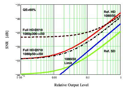
Figure 1 - Noise in Y as a function of output level for 1080i50 output format derived from different input formats at f/10. As a reference the noise is given for the interlace scanned SD and HD cameras. QE is assumed at 60%.
