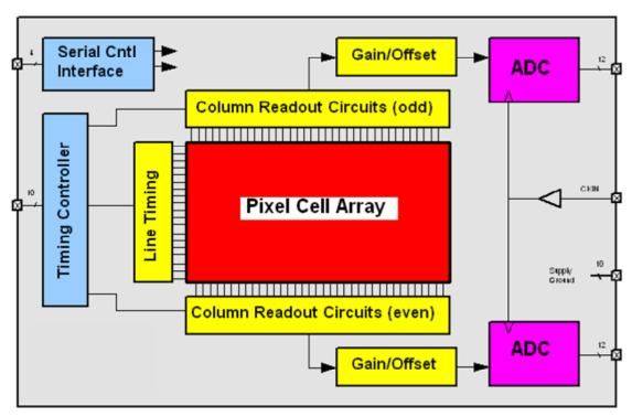
Figure 4 - Block diagram CMOS imager
