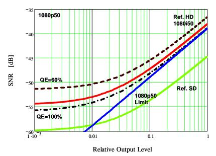
Figure 2 - Noise in Y as a function of output level for 1080p50 at f/10. QE=100% is the theoretical maximum.
