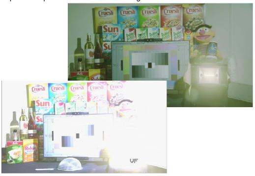
Figure 5 – Image down-left: normal operation, Image upper-right HDR image.
